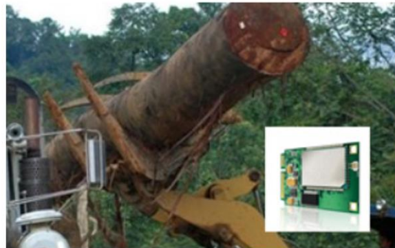
Invisible Track allows an illegally harvested log to send an alert and location once it passes within 20 miles of a cellular network. Courtesy Gemalto
